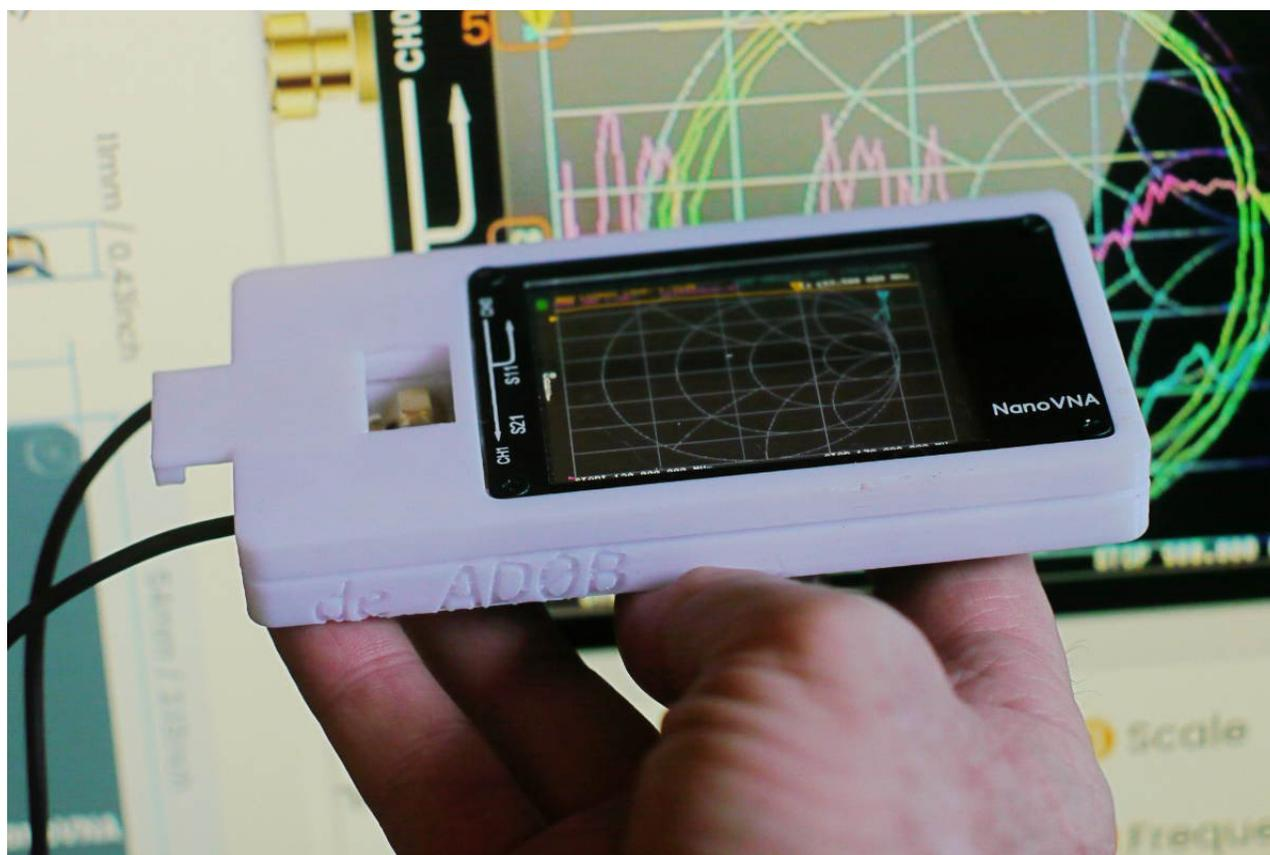
It has coax strain reliefs and a drawer with a sliding cover to hold calibration components. Made from White PETG.
